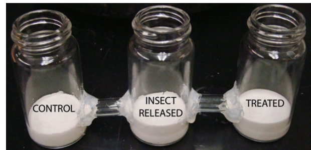
Fig. 1. Choice bioassay setup using three scintillation vials joined by glass tubes. Holes were made in the scintillation vials with a DeWalt 6.4-mm diamond drill bit. One adult female was released in the central arena and had a choice of going to the control berry or to a berry treated with 80 \mu\text{g}/\mu\text{l} ( E,E )- \alpha -farnesene.
